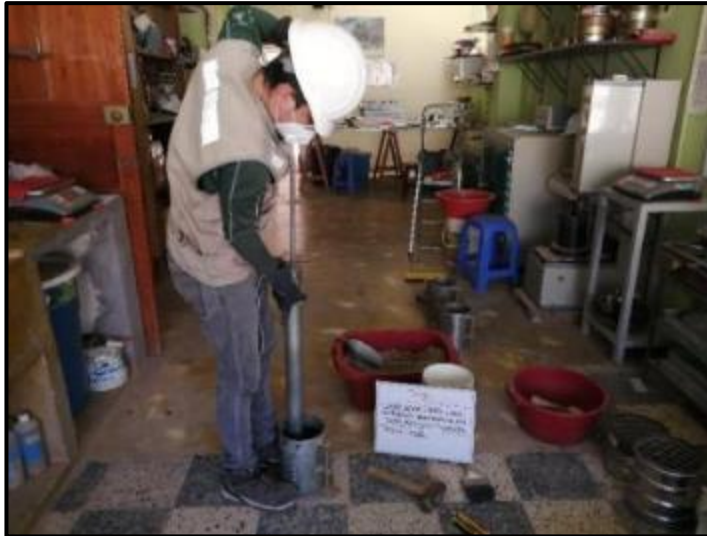
Figura 31 Ensayo de California Bearing Ratio (CBR)
